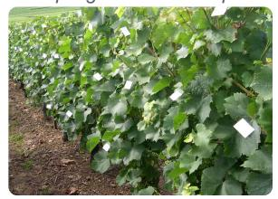
PVC collectors positionned on leaves
